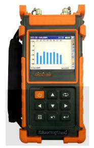
OCC-50 Handheld CWDM Optical Channel Checker is specially designed for CWDM installation, maintenance and troubleshooting, which allows you to measure and monitor power values of up to 18 CWDM channels. OCC-50 can replace high-cost Spectrometers and conduct quick and reliable measurements in all environments. Thanks to its light, compact and sturdy design, OCC-50 is the ideal tool for CWDM installation and maintenance technicians.
